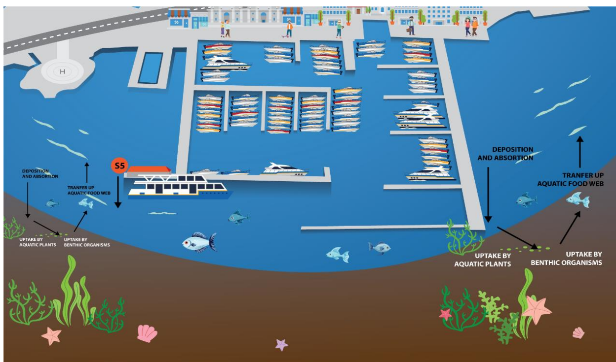
Figure 6. Schematic view of CSM for Porto Montenegro with relationship between a chemical source, exposure pathway and potential receptor
